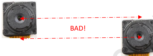
Figure 32- Bad example of camera placement.
