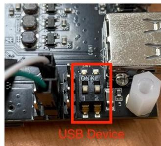
Figure 1-10 Change SW1 Switch to Device
