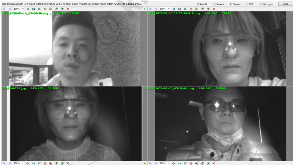
Figure 45 – NIR images, we can see a ring if we turn on the LED
